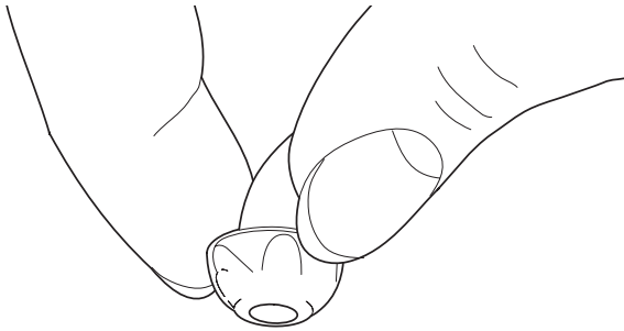
Fig. 10: Replacement of the dome
